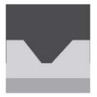
This method for 90° folds may lead to dimensional variations of  $\pm 1.0$ mm and these should be compensated for in the panel size calculations.
