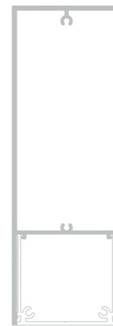
BATTEN OUTER 50mm x 150mm ZCOUTER50/150
